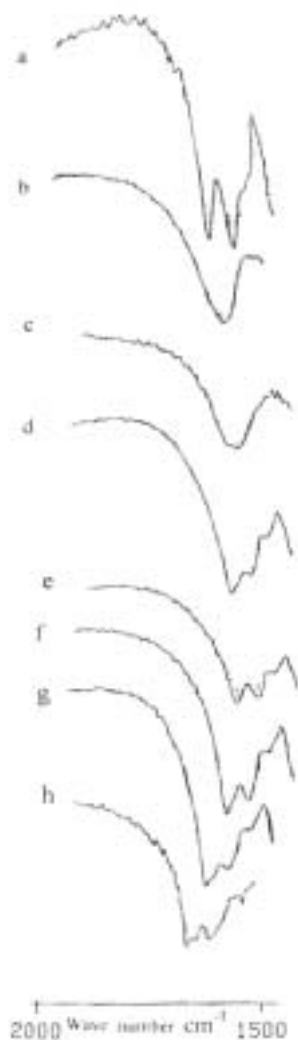
FIGURE 8 FT-IR Spectra of Rutin and Rutin-HP-β-CD Binary Systems: (a) Rutin; (b) HP-β-CD; (c) Rutin-HP-β-CD 1:2 Kn; (d) Rutin-HP-β-CD 1:1 Kn; (e) Rutin-HP-β-CD 1:2 Co; (f) Rutin-HP-β-CD 1:1 Co; (g) Rutin-HP-β-CD 1:2 Pm; (h) Rutin-HP-β-CD 1:1 Pm.
